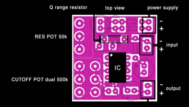
power supply range from 3 volts DC to 15 volts DC
